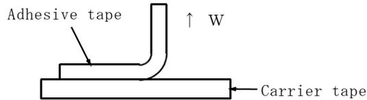
3-6. Tensile test : When pulling a test sample by the force 10N, there shall be no gaps or breakdowns.
