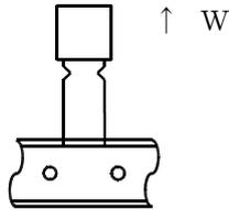
3-7. Moisture resistance : A taped test sample shall be left in a chamber with a temperature of 40°C and RH95% for 96 hours. Then after being left for one hour at room temperature the test sample shall be submitted to a tensile test of item 3.6.
