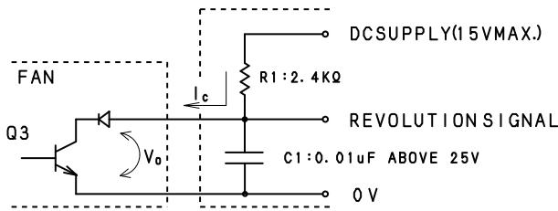
Remark: As for measuring  $V_{OL}$ , it is necessary to put cr low pass filter which is constructed of R1 and C1. The time constant of  $R1 \times C1$  is to be more than 24us such as  $R1=2.4\text{ k}\Omega$   $C1=0.01\text{ }\mu\text{F}$ .
