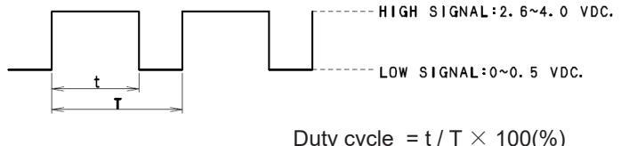
$$\text{Duty cycle} = t / T \times 100\text{ (%)}$$
