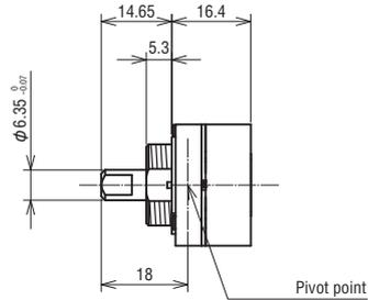
Unless otherwise specified, tolerance:  $\pm 0.4$  (Unit: mm)
