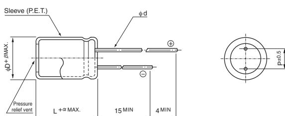
\* In case L > 25 for the φD dia. unit, lead dia. φ d = 0.8mm.
