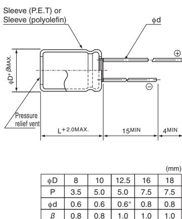
※ In case L &gt; 25 for the φ12.5 dia. unit, lead dia. φ d = 0.8mm.
