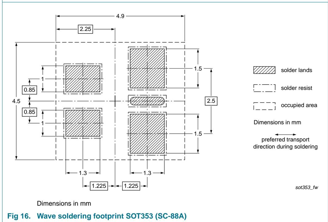
**Fig 16. Wave soldering footprint SOT353 (SC-88A)**
