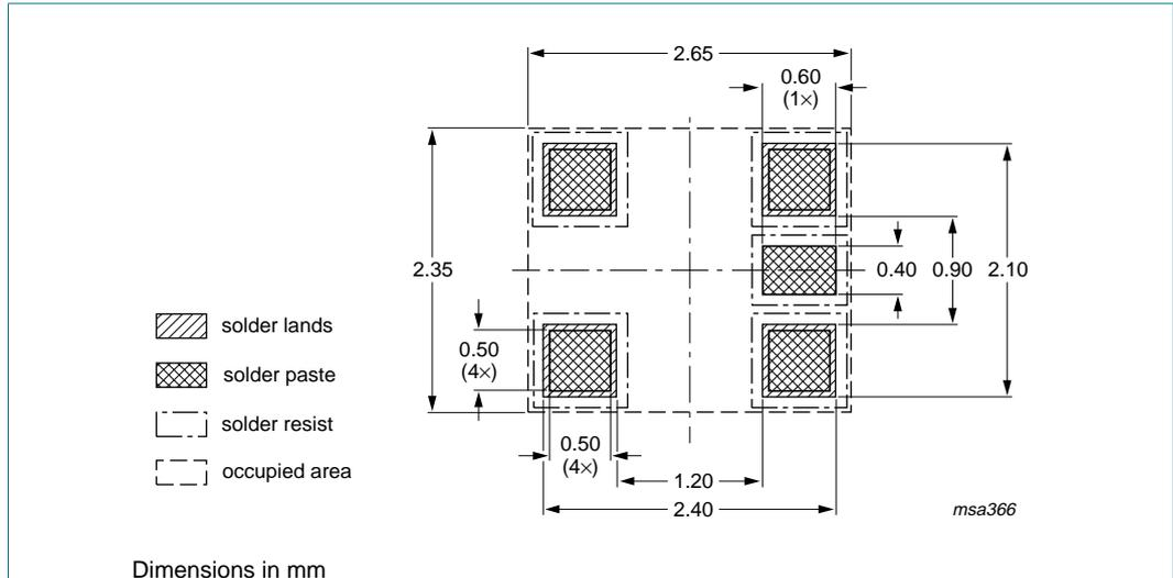
**Fig 15. Reflow soldering footprint SOT353 (SC-88A)**
