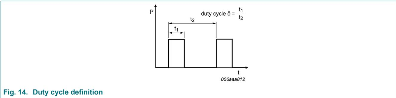
Fig. 14. Duty cycle definition
