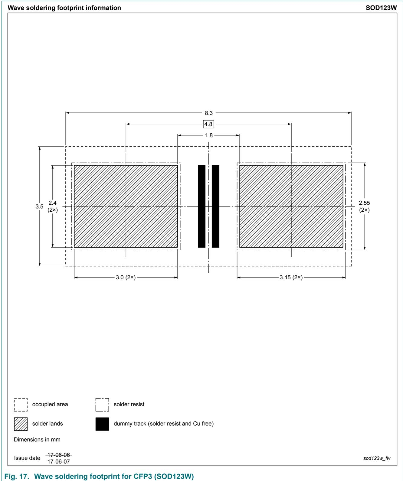
**Fig. 17. Wave soldering footprint for CFP3 (SOD123W)**
