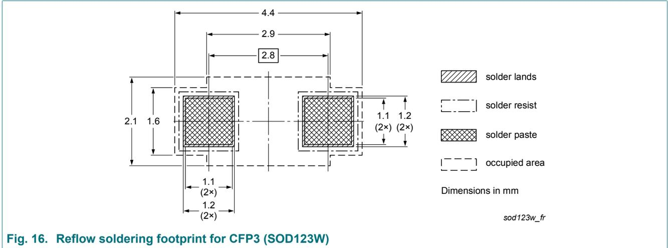
Fig. 16. Reflow soldering footprint for CFP3 (SOD123W)
