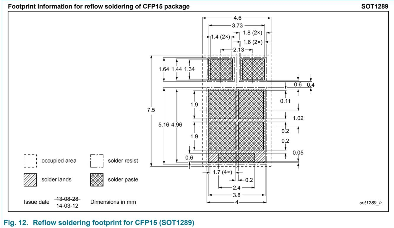
Fig. 12. Reflow soldering footprint for CFP15 (SOT1289)
