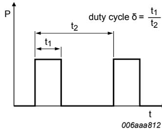
Fig. 10. Duty cycle definition
