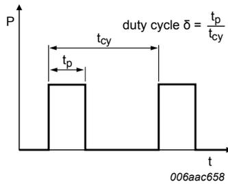
Fig. 13. Duty cycle definition
