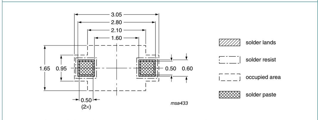
Reflow soldering is the only recommended soldering method.
