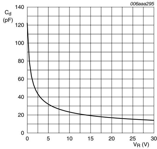
$T_{amb} = 25\text{ }^\circ\text{C}; f = 1\text{ MHz}$
