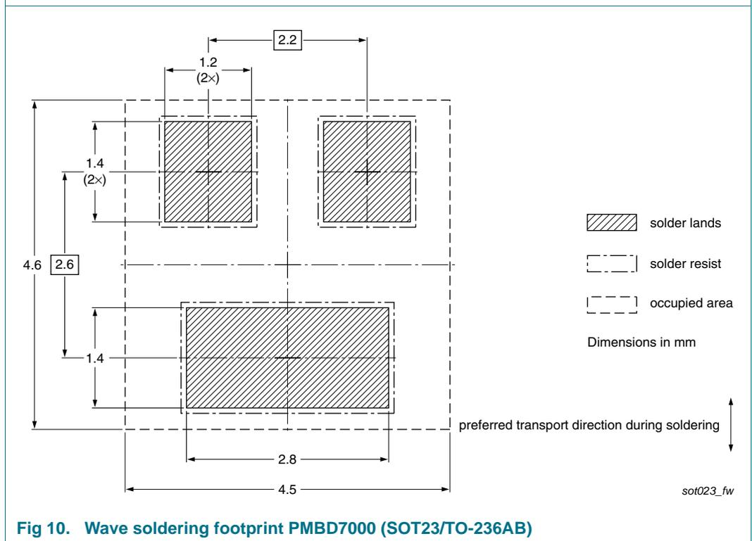
**Fig 10. Wave soldering footprint PMBD7000 (SOT23/TO-236AB)**
