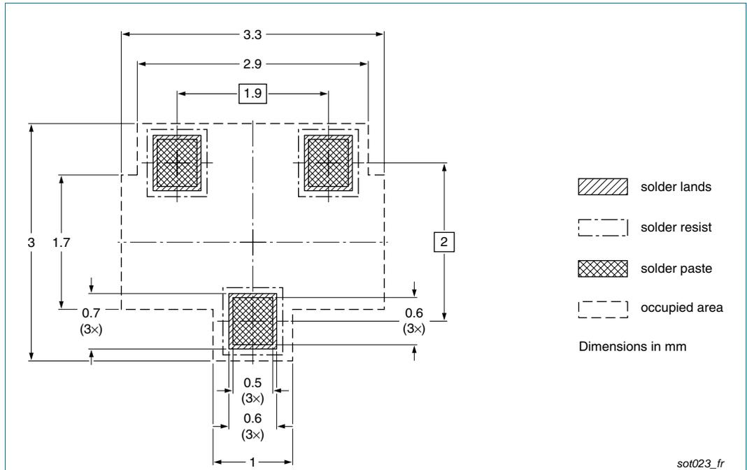
**Fig 9. Reflow soldering footprint PMBD7000 (SOT23/TO-236AB)**
