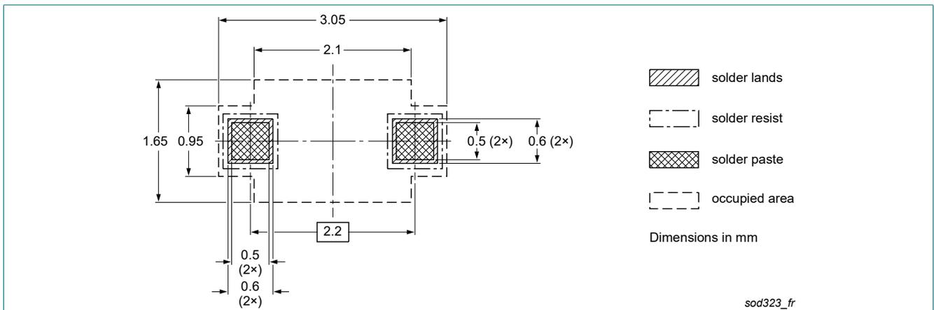
Fig. 7. Reflow soldering footprint for SOD323
