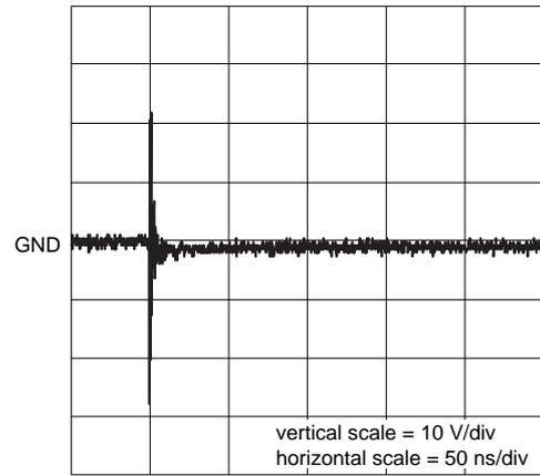
clamped -1 kV ESD voltage waveform (IEC61000-4-2 network)
