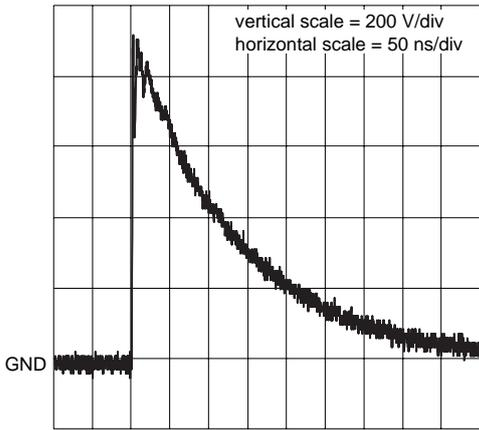
unclamped +1 kV ESD voltage waveform (IEC61000-4-2 network)
