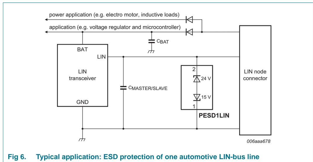
**Fig 6. Typical application: ESD protection of one automotive LIN-bus line**
