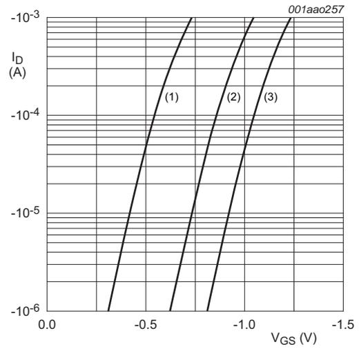
$T_j = 25\text{ °C}; V_{DS} = -5\text{ V}$
