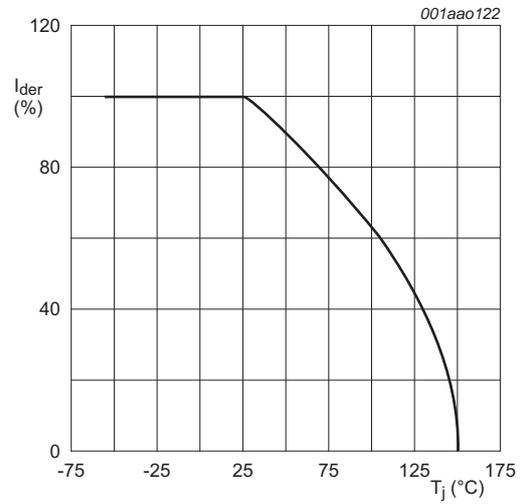
$$I_{der} = \frac{I_D}{I_{D(25^{\circ}\text{C})}} \times 100\%$$
