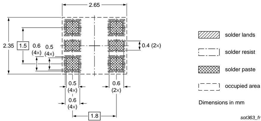
**Fig 19. Reflow soldering footprint for SOT363 (SC-88)**
