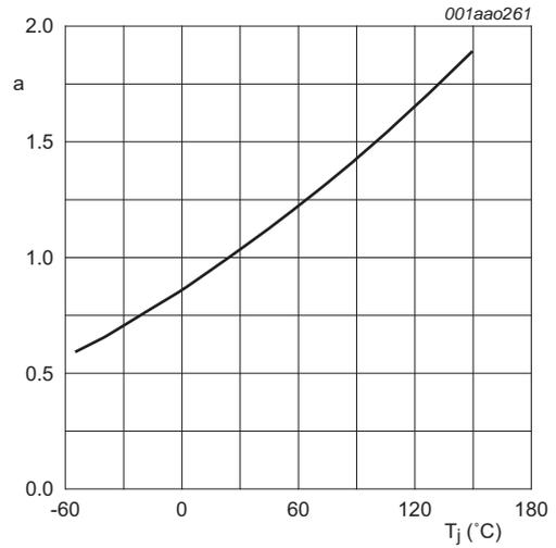
$$a = \frac{R_{DS(on)}}{R_{DS(on)@25^\circ\text{C}}}$$
