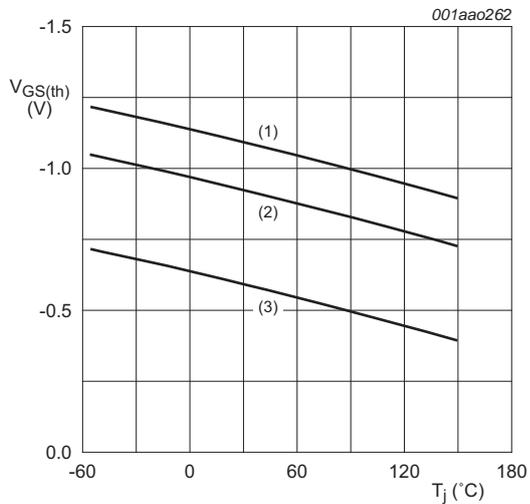
$I_D = -0.25\text{ mA}; V_{DS} = V_{GS}$
