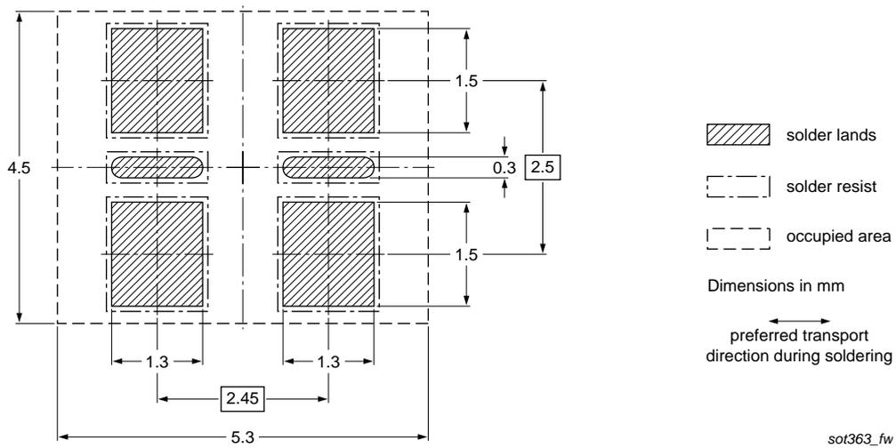
**Fig 20. Wave soldering footprint for SOT363 (SC-88)**
