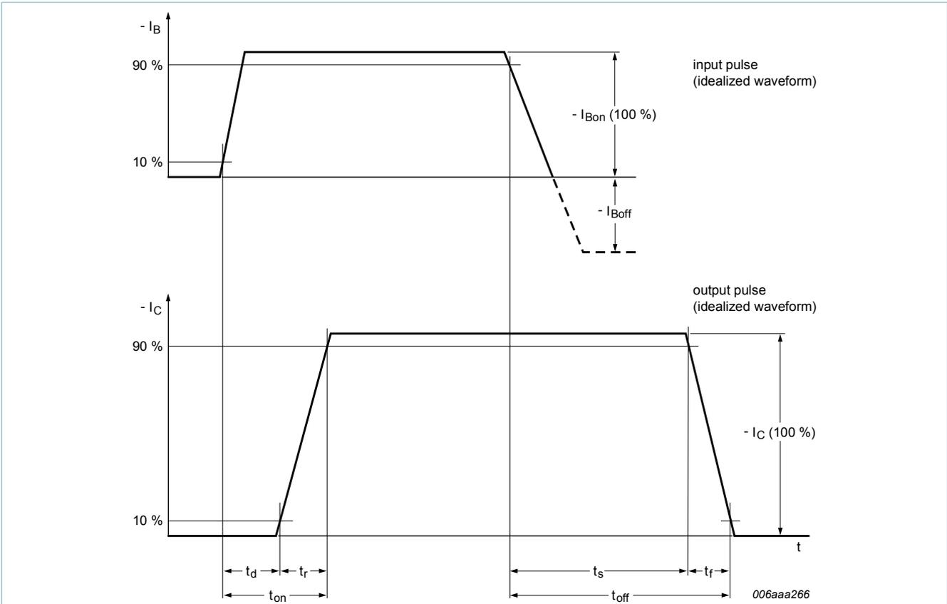
Fig. 16. TR2 (PNP): Transistor switching time definition
