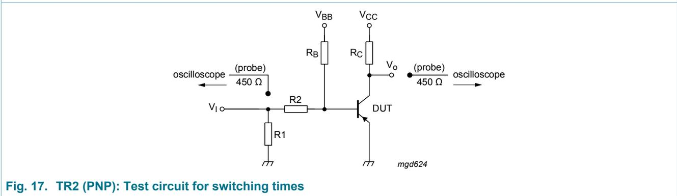
Fig. 17. TR2 (PNP): Test circuit for switching times
