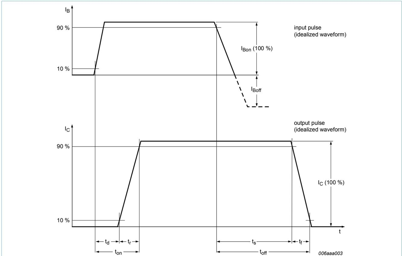
Fig. 14. TR1 (NPN): Transistor switching time definition
