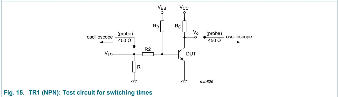
Fig. 15. TR1 (NPN): Test circuit for switching times
