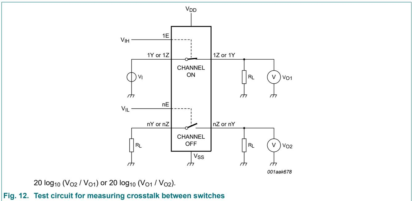
Fig. 12. Test circuit for measuring crosstalk between switches
