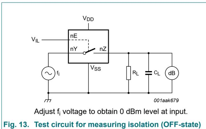
Fig. 13. Test circuit for measuring isolation (OFF-state)
