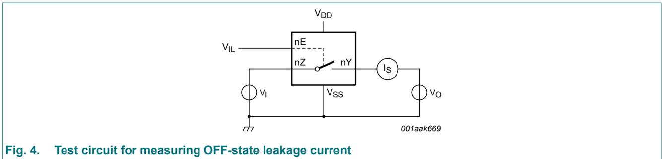
**Fig. 4. Test circuit for measuring OFF-state leakage current**
