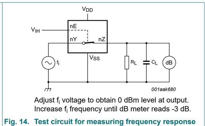
Fig. 14. Test circuit for measuring frequency response
