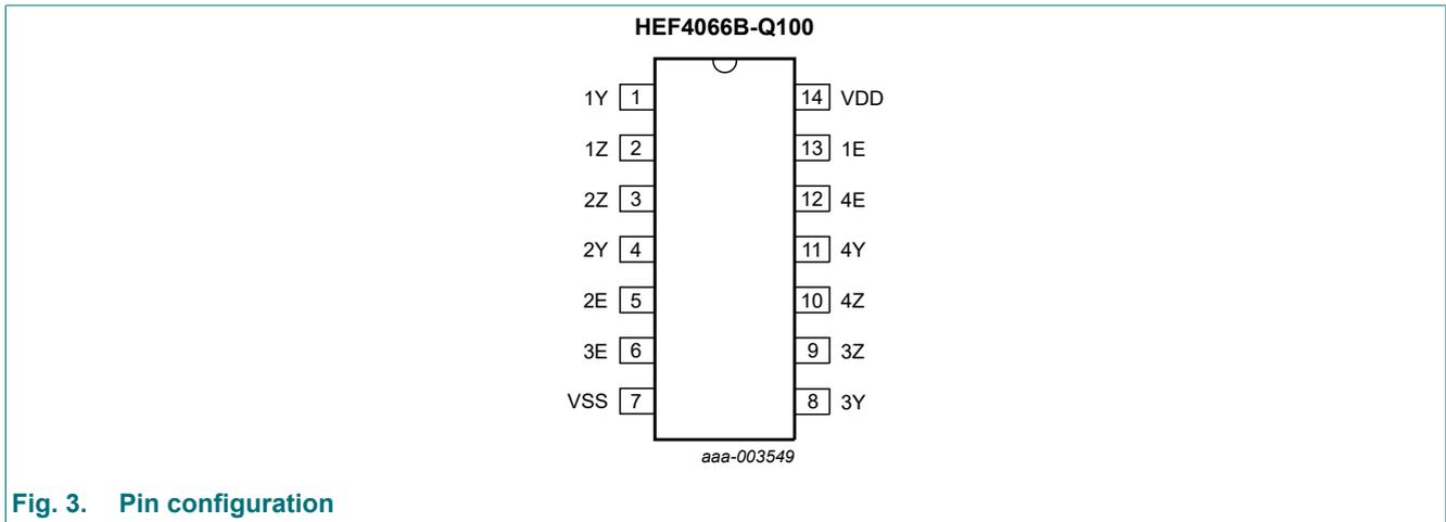
Fig. 3. Pin configuration
