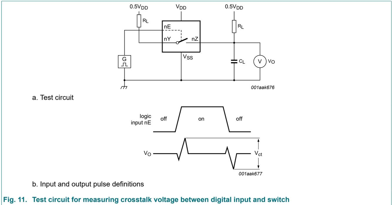
Fig. 11. Test circuit for measuring crosstalk voltage between digital input and switch
