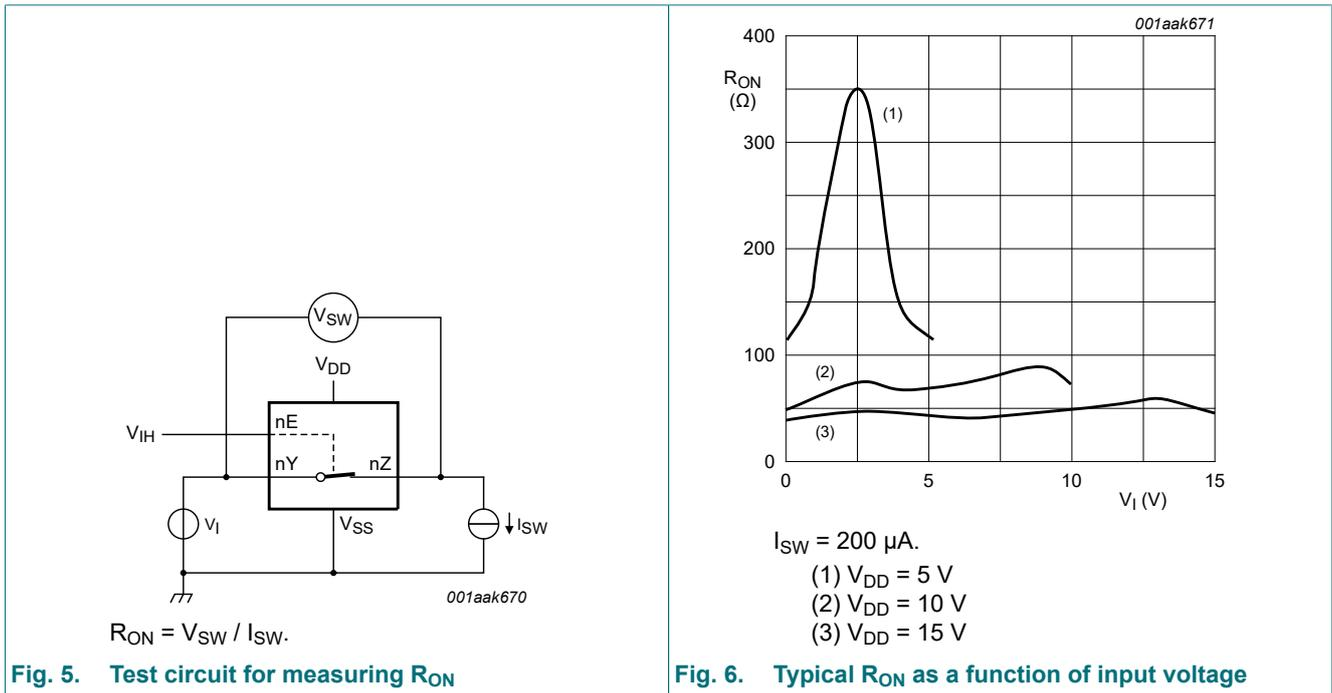
Fig. 5. Test circuit for measuring R<sub>ON</sub>
