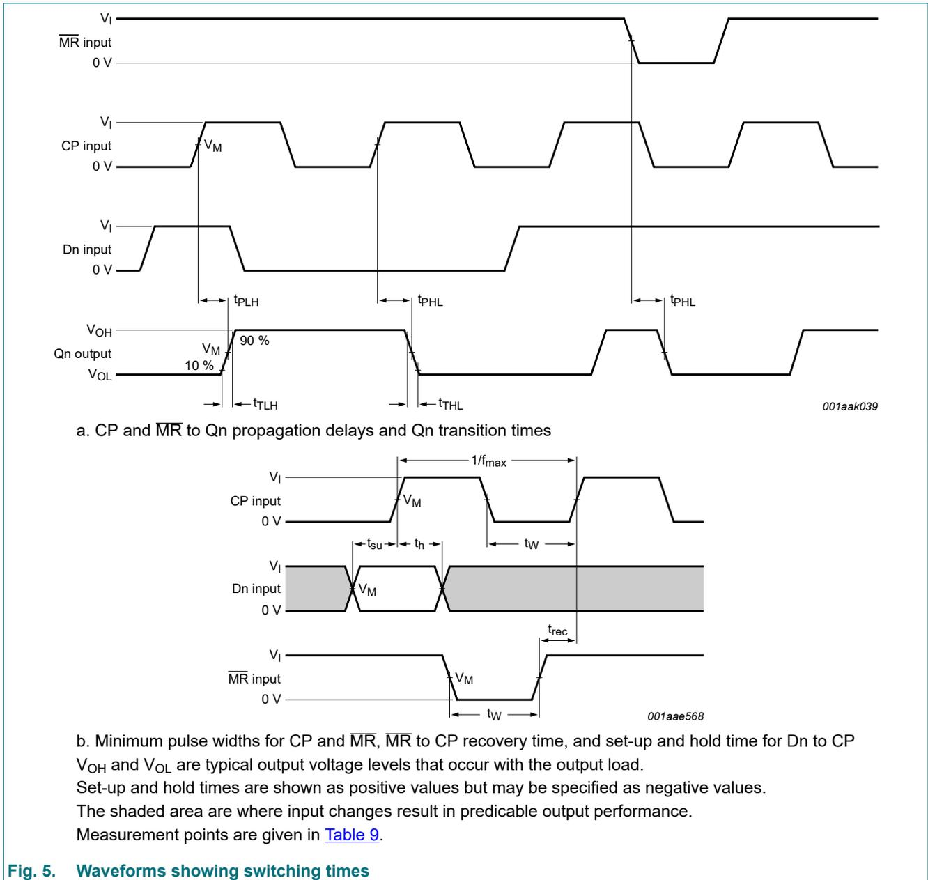
**Fig. 5. Waveforms showing switching times**
