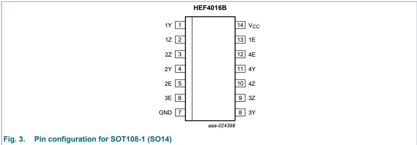
Fig. 3. Pin configuration for SOT108-1 (SO14)
