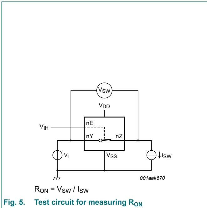
Fig. 5. Test circuit for measuring  $R_{ON}$
