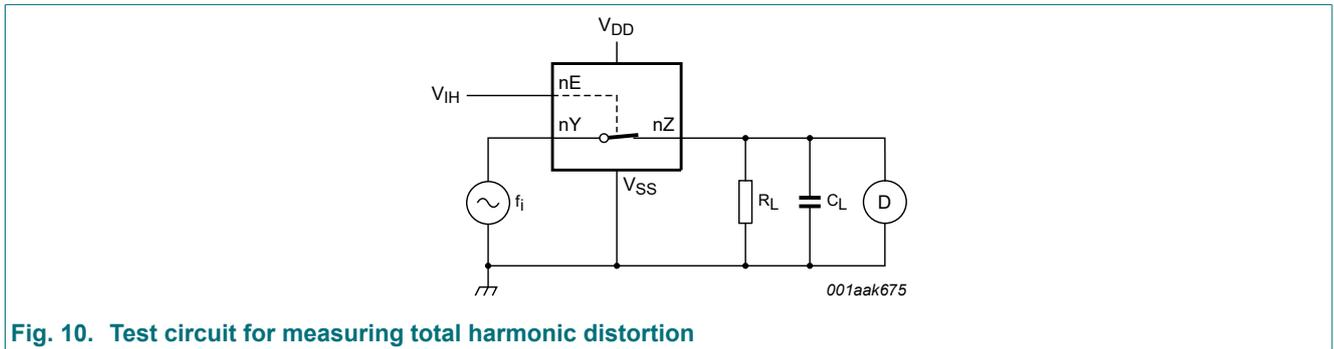
Fig. 10. Test circuit for measuring total harmonic distortion
