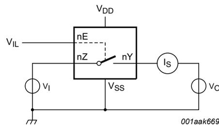
**Fig. 4. Test circuit for measuring OFF-state leakage current**
