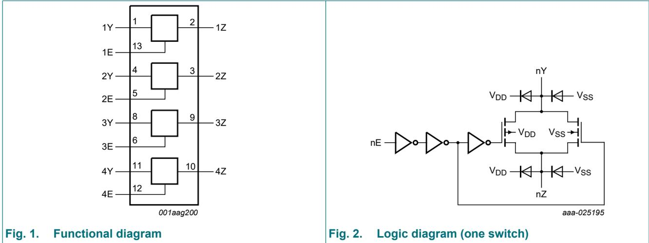
Fig. 1. Functional diagram
