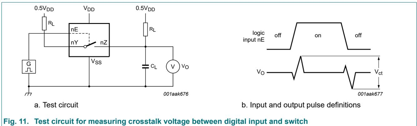
Fig. 11. Test circuit for measuring crosstalk voltage between digital input and switch
