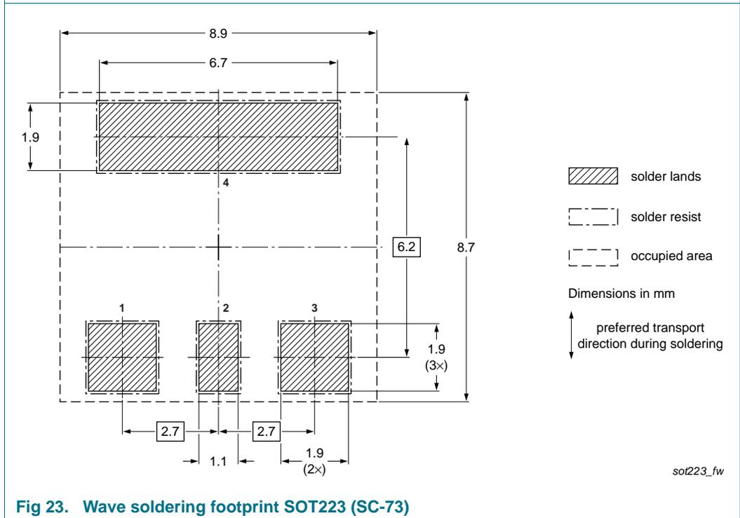
Fig 23. Wave soldering footprint SOT223 (SC-73)
