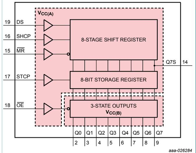
Figure 2. Functional diagram
