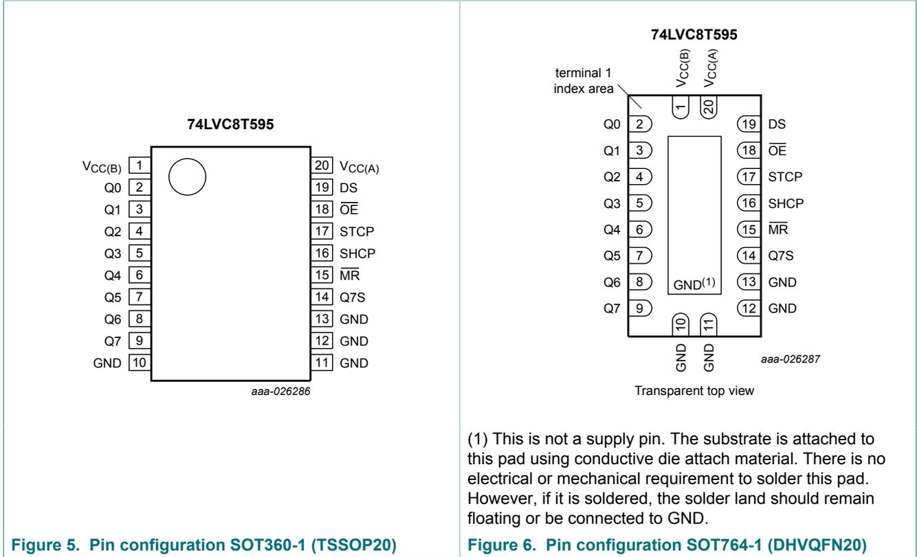
Figure 5. Pin configuration SOT360-1 (TSSOP20)
