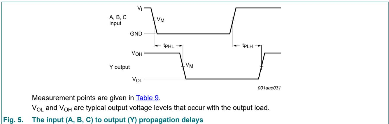
**Fig. 5. The input (A, B, C) to output (Y) propagation delays**
