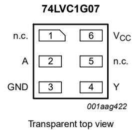
Fig. 5. Pin configuration SOT886, SOT1115 and SOT1202 (XSON6)
