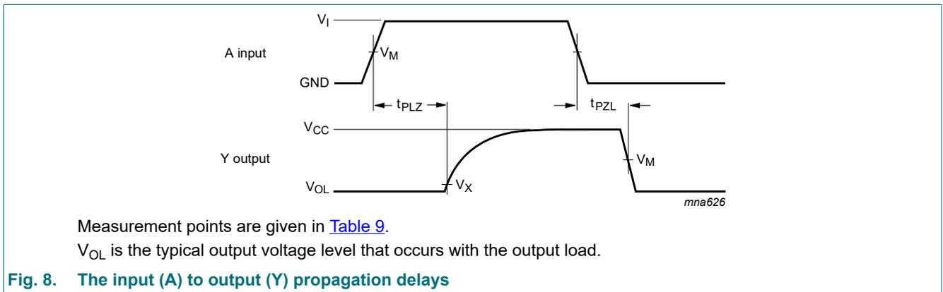
**Fig. 8. The input (A) to output (Y) propagation delays**
