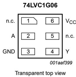
Fig. 6. Pin configuration SOT1115 and SOT1202 (XSON6)
