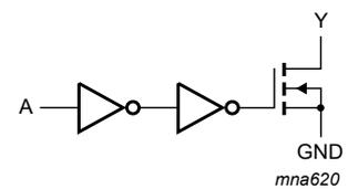
Fig. 3. Logic diagram
