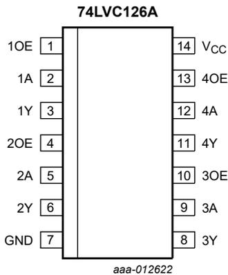
Fig. 4. Pin configuration SOT108-1 (SO14) and SOT402-1 (TSSOP14)
