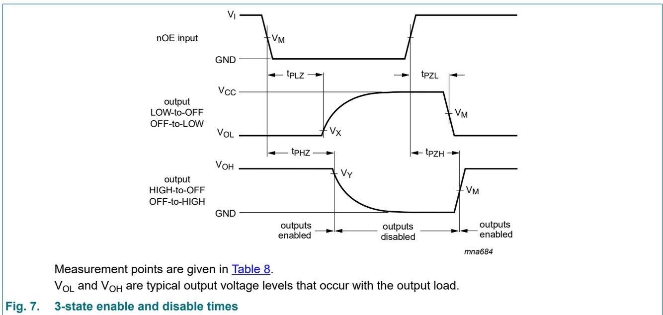
Quad buffer/line driver with 5 V tolerant input/outputs; 3-state
