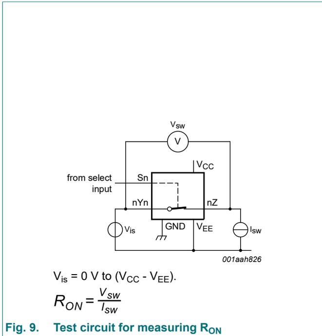
Fig. 9. Test circuit for measuring  $R_{ON}$
