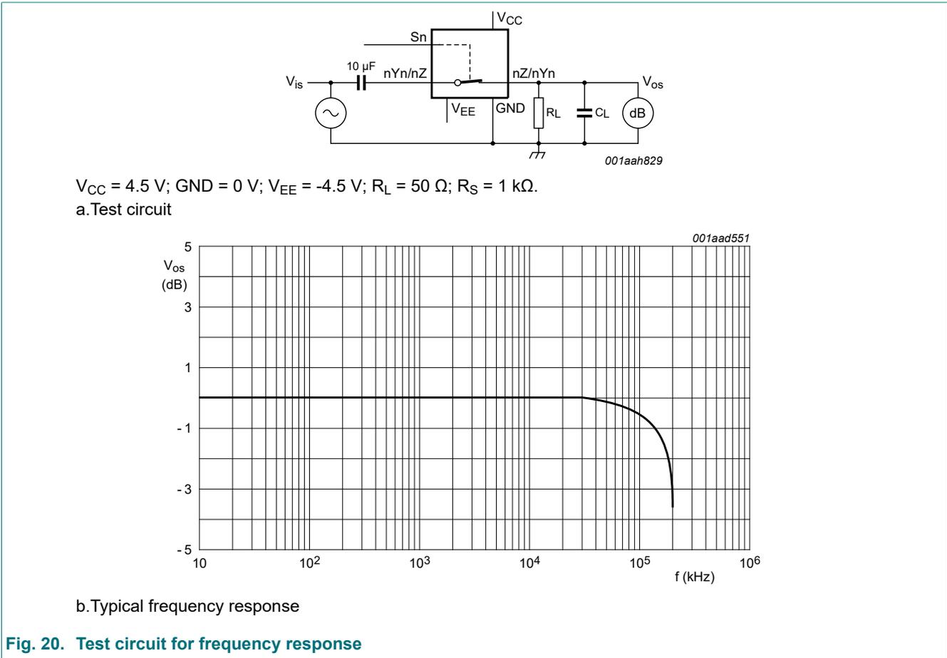
Fig. 20. Test circuit for frequency response
