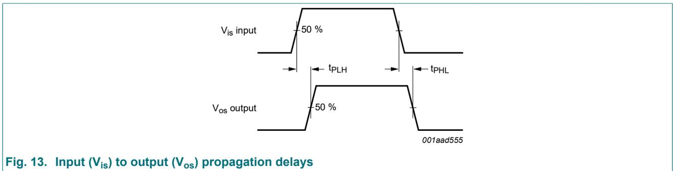
Fig. 13. Input (V<sub>is</sub>) to output (V<sub>os</sub>) propagation delays
