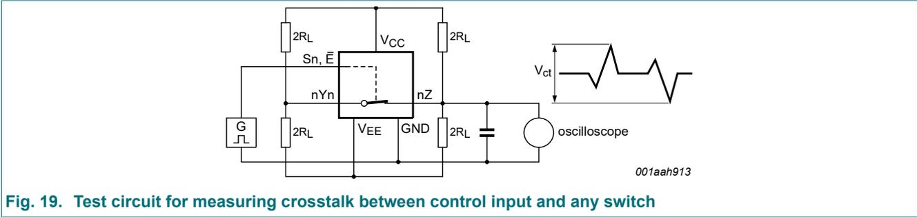
Fig. 19. Test circuit for measuring crosstalk between control input and any switch
