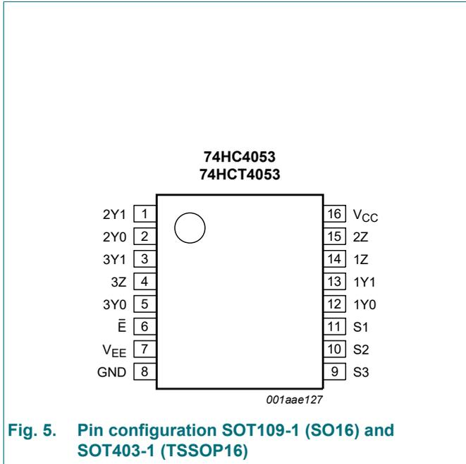
Fig. 5. Pin configuration SOT109-1 (SO16) and SOT403-1 (TSSOP16)
