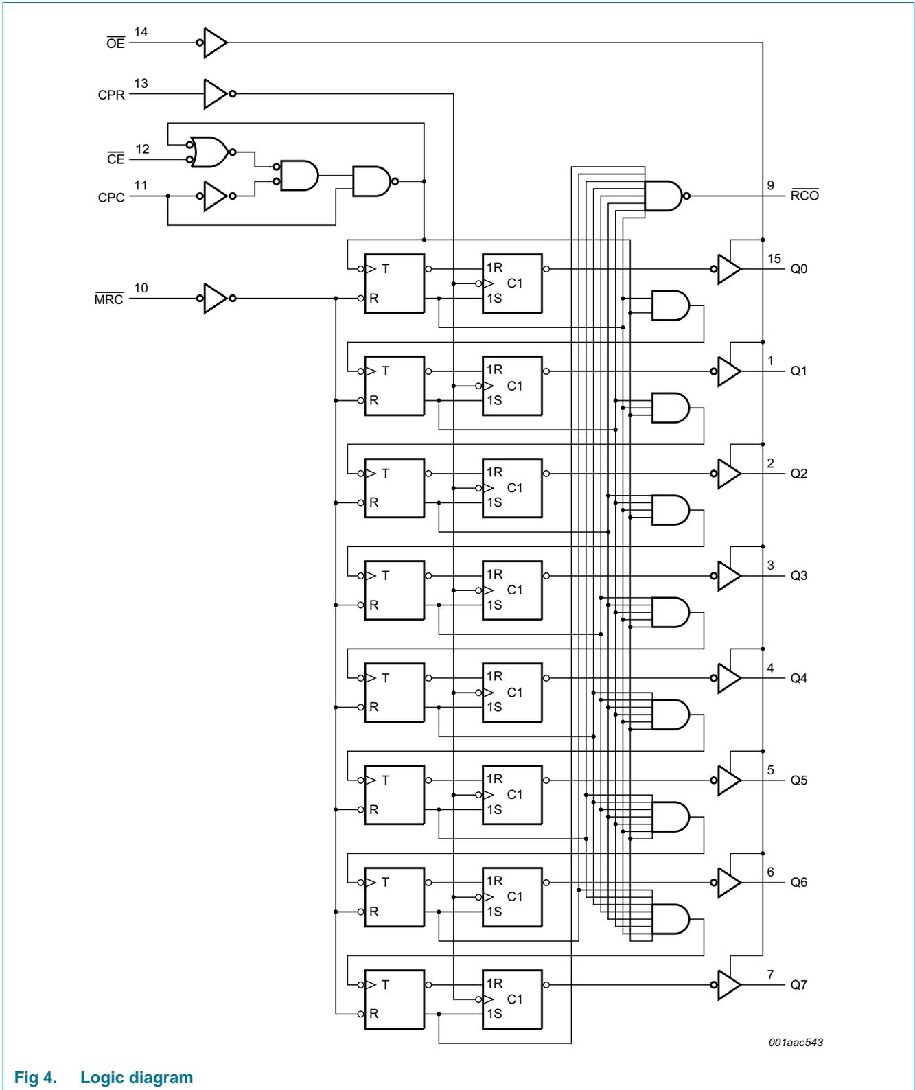
Fig 4. Logic diagram
