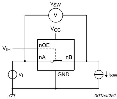
$R_{ON} = V_{SW} / I_{SW}$ .
