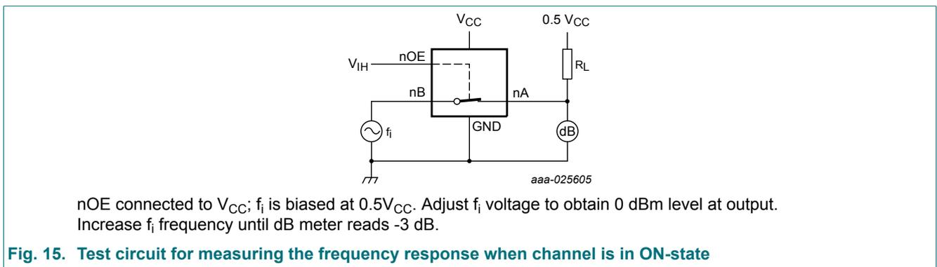
**Fig. 15. Test circuit for measuring the frequency response when channel is in ON-state**
