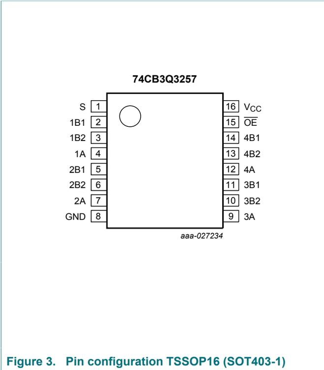
Figure 3. Pin configuration TSSOP16 (SOT403-1)
