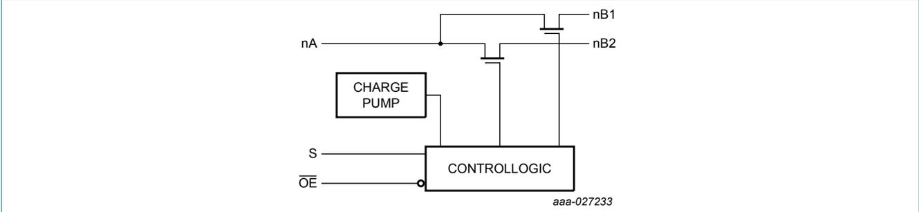
Figure 2. Logic diagram (one switch)
