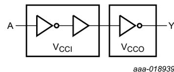
Fig 2. Logic diagram
