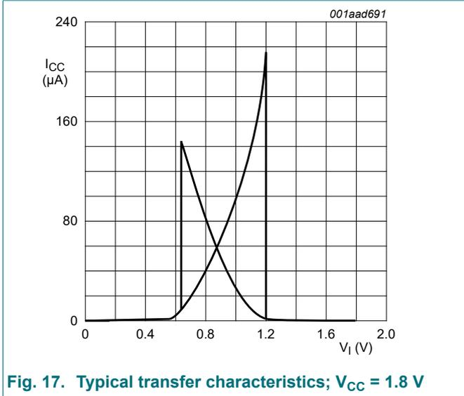
Fig. 17. Typical transfer characteristics;  $V_{CC} = 1.8\text{ V}$
