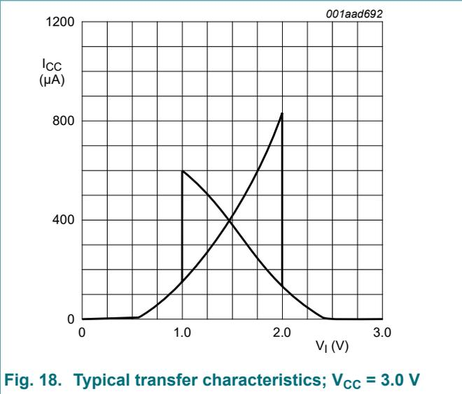
Fig. 18. Typical transfer characteristics;  $V_{CC} = 3.0\text{ V}$
