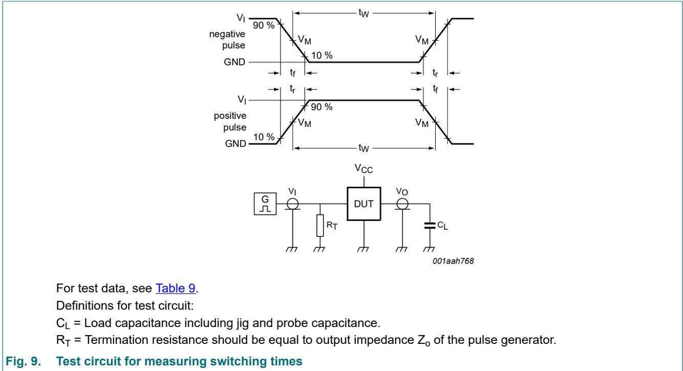
Fig. 9. Test circuit for measuring switching times
