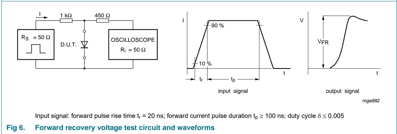
**Fig 6. Forward recovery voltage test circuit and waveforms**
