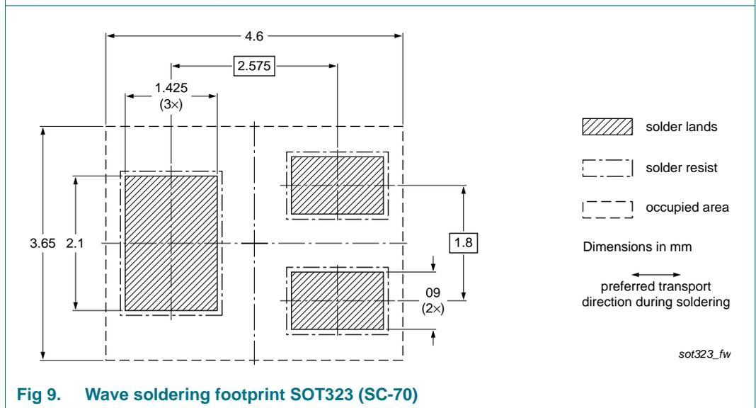
Fig 9. Wave soldering footprint SOT323 (SC-70)
