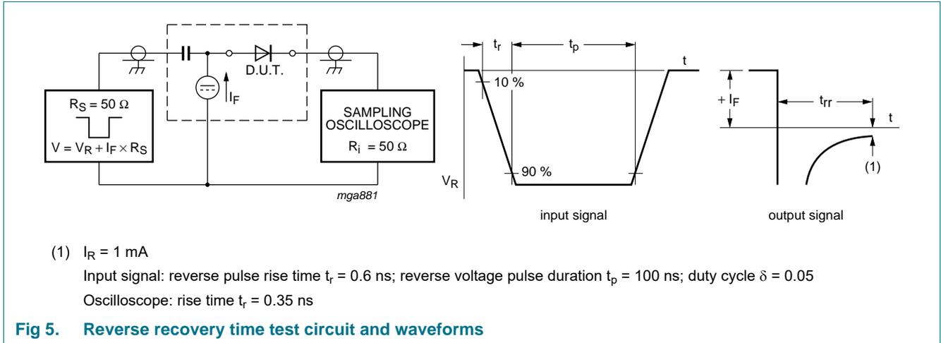
**Fig 5. Reverse recovery time test circuit and waveforms**
