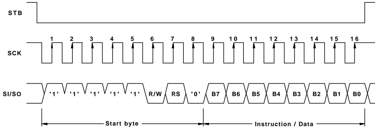
**Figure 11.** Typical Synchronous Serial Interface Write Cycle
