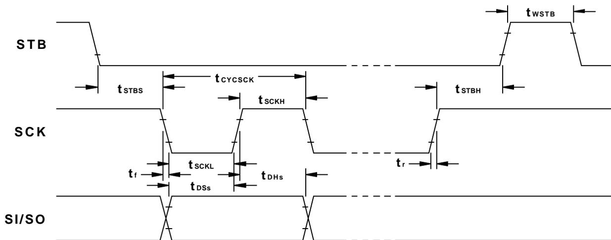
**Figure 7.** Synchronous Serial Interface Write Cycle Timing
