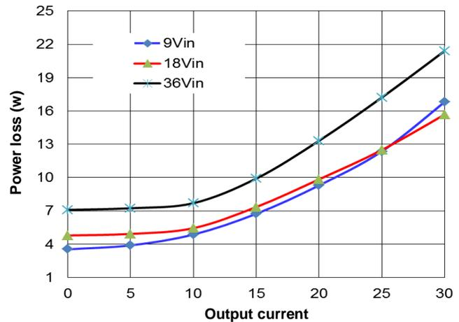
Figure 2. Power Loss vs. Load Current (25°C)
