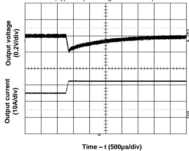
Figure 6. Transient Load Response
