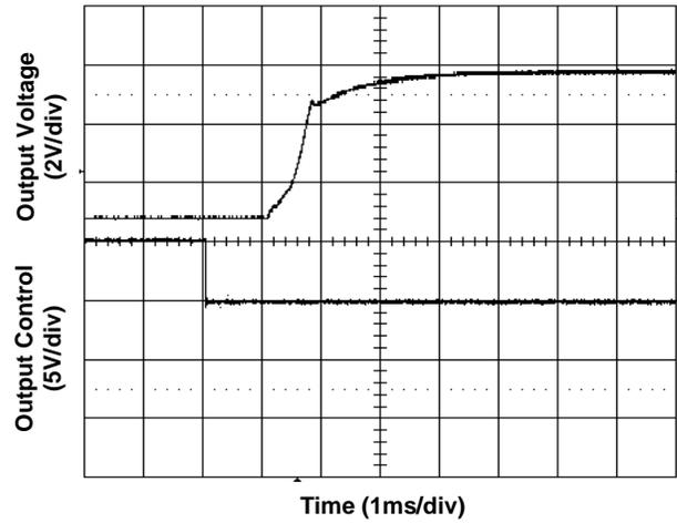
Figure 4. Start-Up from Enable Control
