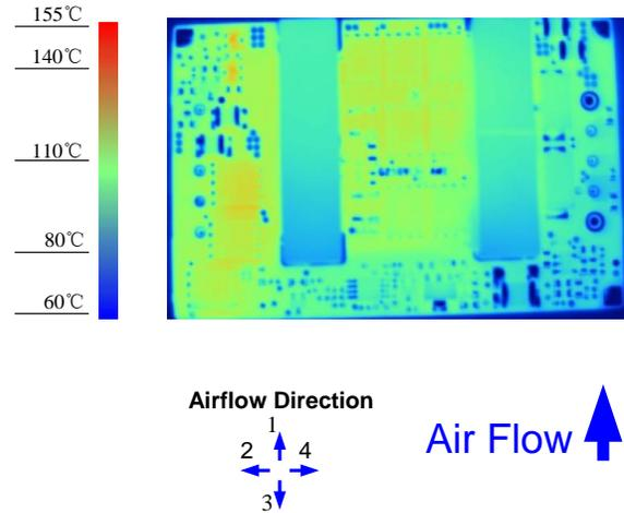
**Figure 9.** Thermal Image for Airflow Direction 1 (25.5A output, 55°C ambient, 200 LFM, typical  $V_{in}$ , open frame, unit soldered onto a fixture board.)
