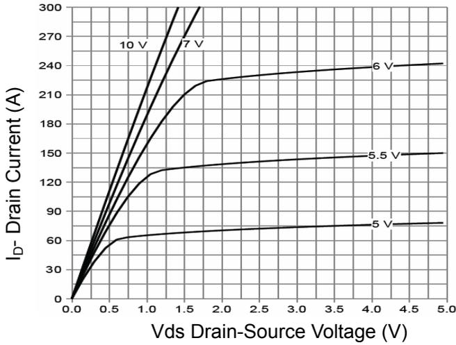
Figure 1 Output Characteristics
