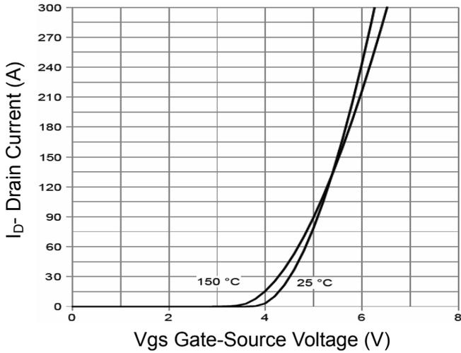
Figure 2 Transfer Characteristics
