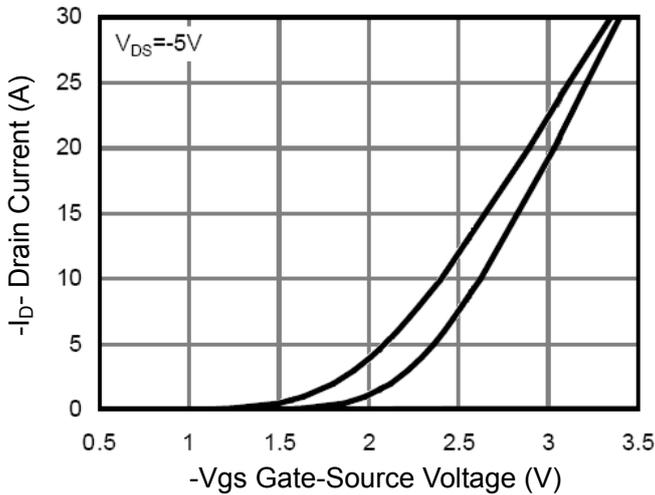
Figure 2 Transfer Characteristics
