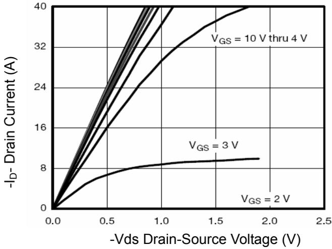
Figure 1 Output Characteristics
