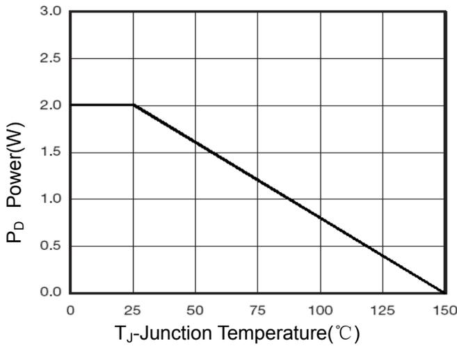
Figure 3 Power Dissipation
