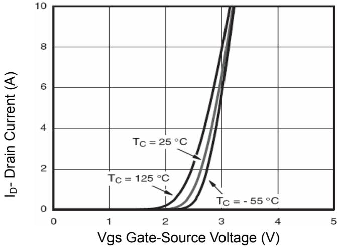
Figure 7 Transfer Characteristics
