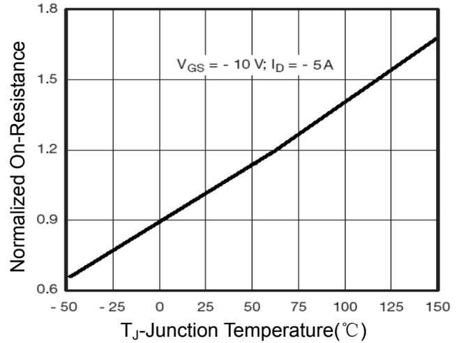
Figure 8 Drain-Source On-Resistance
