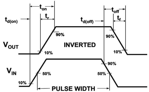
Figure 2: Switching Waveforms
