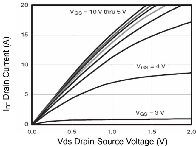
Figure 5 Output Characteristics
