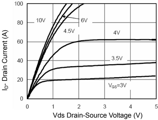
Figure 1 Output Characteristics
