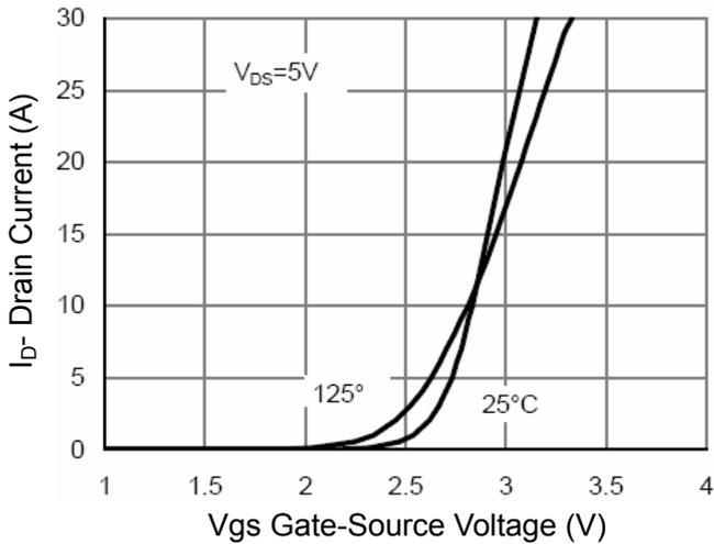
Figure 2 Transfer Characteristics
