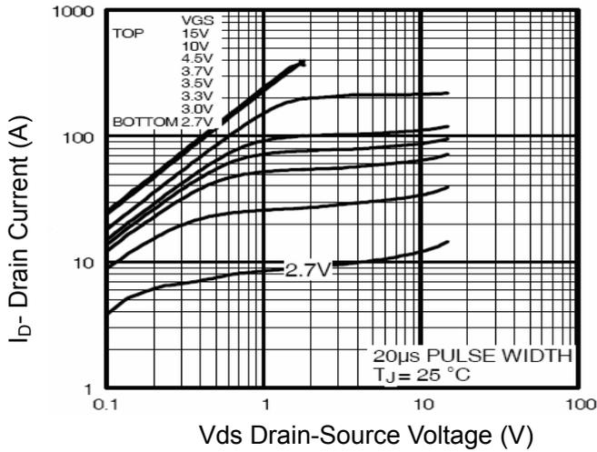
Figure 1 Output Characteristics
