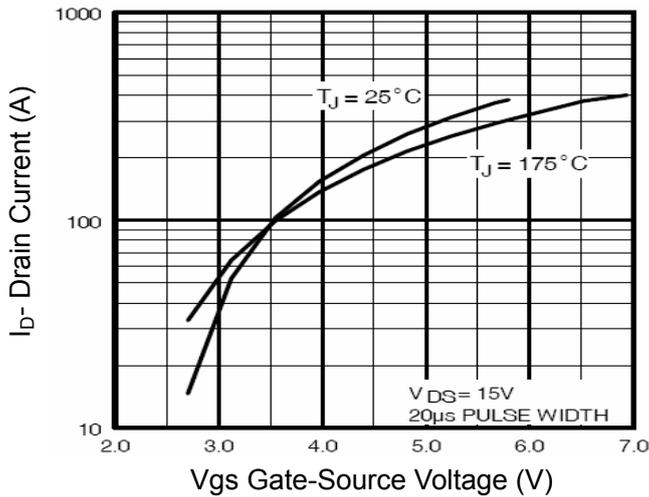
Figure 2 Transfer Characteristics
