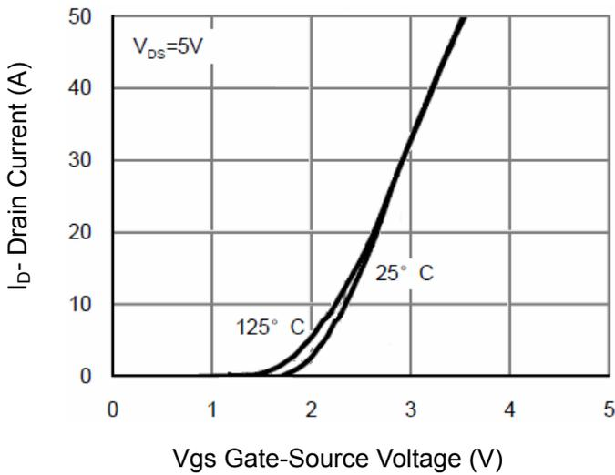
**Figure 2 Transfer Characteristics**
