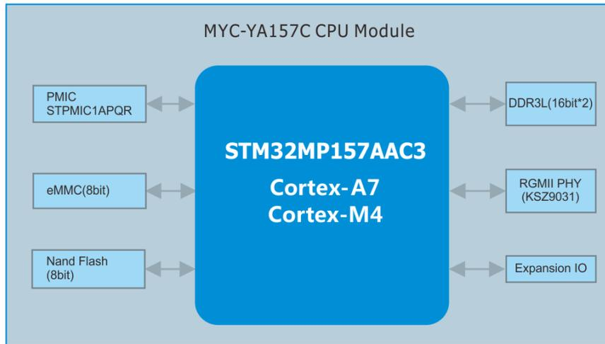
Figure 1-8 MYC-YA157C CPU Module Function Block Diagram
