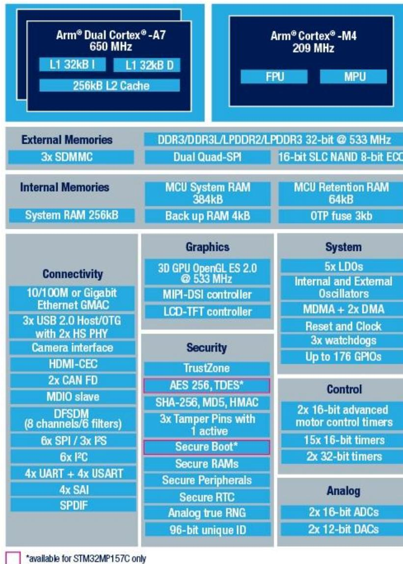
Figure 1-5 STM32MP157 Block Diagram
