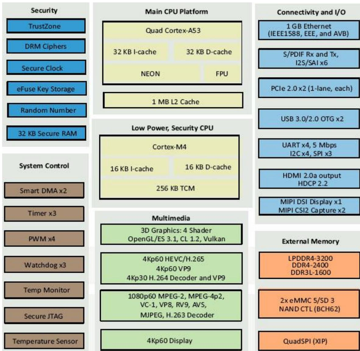
Figure 1-5 i.MX 8M System Block Diagram
