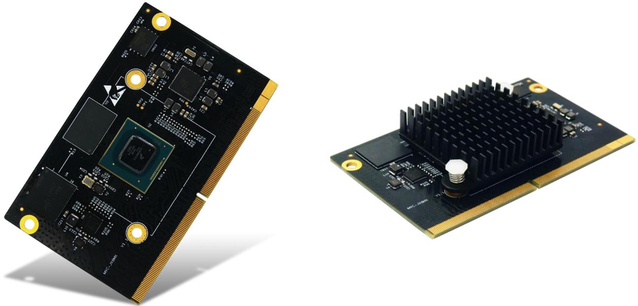
Figure 1-1 MYC-JX8MX CPU Module (delivered with installed heatsink by default)
