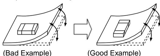
Locate chip horizontal to the direction in which stress acts.
