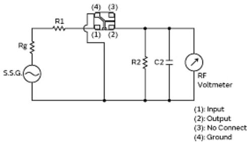
R1+Rg=R2=Input/Output Impedance, Rg=50Ω
