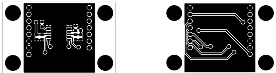
Figure 2. TOP (left) and BOTTOM (right) layout of SCA3300 PCB (aspect ratio not 1:1).
