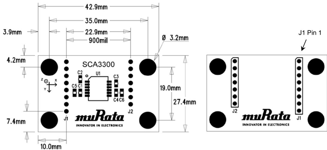
Figure 3. TOP (left) and BOTTOM (right) view assembly drawings for SCA3300 PCB (aspect ratio not 1:1).
