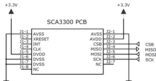
Figure 1. SCA3300 PCB pinout and external connections.
