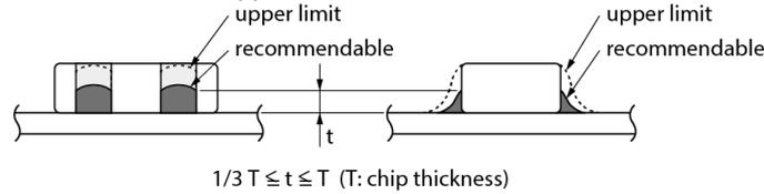
An increased solder volume increases mechanical stress on the product. Exceeding solder volume may cause the failure of mechanical or electrical performance.
