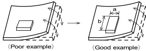
(2) Components location on PCB separation
