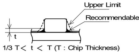
Accordingly increasing the solder volume, the mechanical stress to product is also increased. Excessive solder volume may cause the failure of mechanical or electrical performance.
