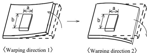
Products(warping direction 1, warping direction 2) shall be located carefully so that products are not subject to the mechanical stress due to warping the board. Because they may be subjected the mechanical stress in order of warping direction 1>warping direction 2.
