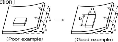
Products shall be location the sideways Direction (Length : a<b) to the machanical Stress.
