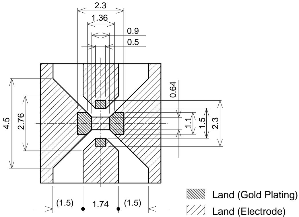
(Note) ·The material of PWB is the epoxy resin of glass fabric base. ( $\epsilon_r=4.8$ ). Thickness is 1.0mm.
