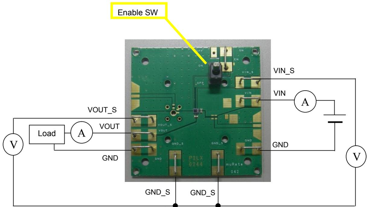
The enable switch has three positions.
